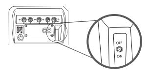
IF THE SWITCH IS NOT VISIBLE PUSH TOWARDS THE SOLAR PANEL
